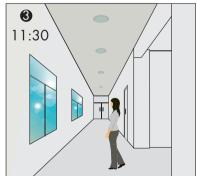
The light turns off completely whenever natural light reaches above pre-set daylight threshold, even with presence.
